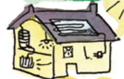
LA CHALEUR PRODUITE PAR LES PANNEAUX PHOTOVOLTAÏQUES EST RÉCUPÉRÉE SOIT PAR UNE VENTILATION SOIT PAR UN FLUIDE, ET RENVOYÉE VERS LE BALLON D'EAU CHAUDE OU LE CHAUFFAGE.
